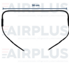
RESISTENCIA "U" MABE CHICA 38CMS 120V/280W C/FUSIBLE TERMINAL ESPADA
